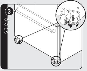
To lower the front of the refrigerator, turn the leveler foot screw counterclockwise. **Note:** Having someone push against the top of the refrigerator takes some weight off the leveler foot. This makes it easier to turn the levelers. It may take several turns of the leveler foot screw to adjust the tilt of the refrigerator.
